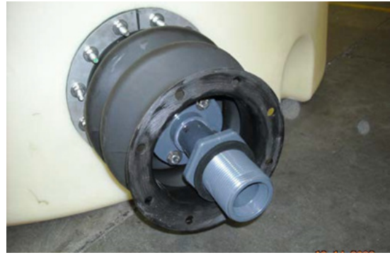
INSTALL BELLOWS HOUSING AND 8" SPLIT RING USING THE PROVIDED HARDWARE. NOTE: AFTER ASSEMBLY IS GLUED REMOVE GASKET FROM BHF AND CHECK WITH A STRAIGHT EDGE. TO ENSURE ALL SEALING SURFACES ARE ON THE SAME PLANE.
