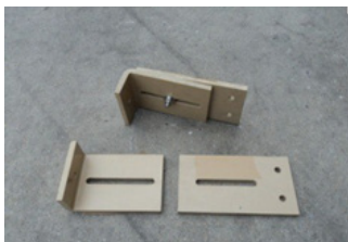
Bolt the mounting bracket to the adjustment plate
